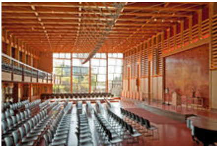
This photo show the new 500-seat atrium auditorium, featuring abundant natural daylight and ventilation. A sunscreen reduces glare from early morning sunlight. - Photo Credit: The Kubala Washatko Architects, Inc. / Zane Williams
