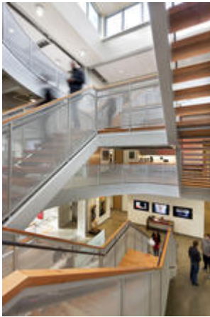
A central core with a motorized roof monitor above aids in the stack ventilation - Photo Credit: Lara Swimmer
